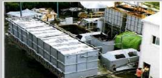
DAF Operation: Separation & Clarification for the factory influent and separating bio-sludge from biological reactor. Courtesy PepsiCo, Frito-Lay International
